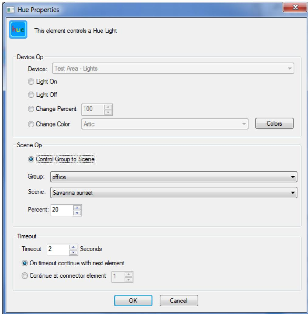
As you can see there are device and group operations. A device can be controlled on, off, to a level, or to a color.
