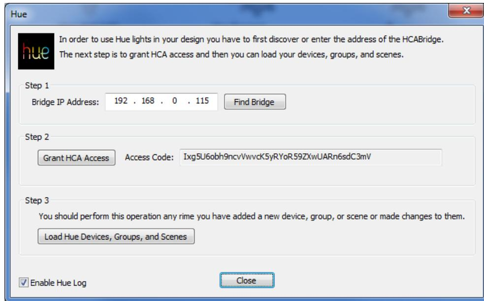
Follow the steps in the dialog. The “Find” operation works only if the Hue Bridge has been powered on for a while. The “Grant HCA Access” asks you to tap the button on the top of the Hue Bridge and then it will authorize HCA and generate an access code which the dialog displays.
