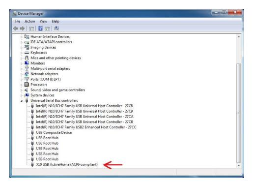
Right click on the "X10 USB ActiveHome (ACPI-Compliant)" line and select "Uninstall" from the popup menu. A popup dialog will confirm that you want to do this. **Make sure** that you check the "Delete the driver software for this device" option and then press OK. The device manager refreshes the display when done.
