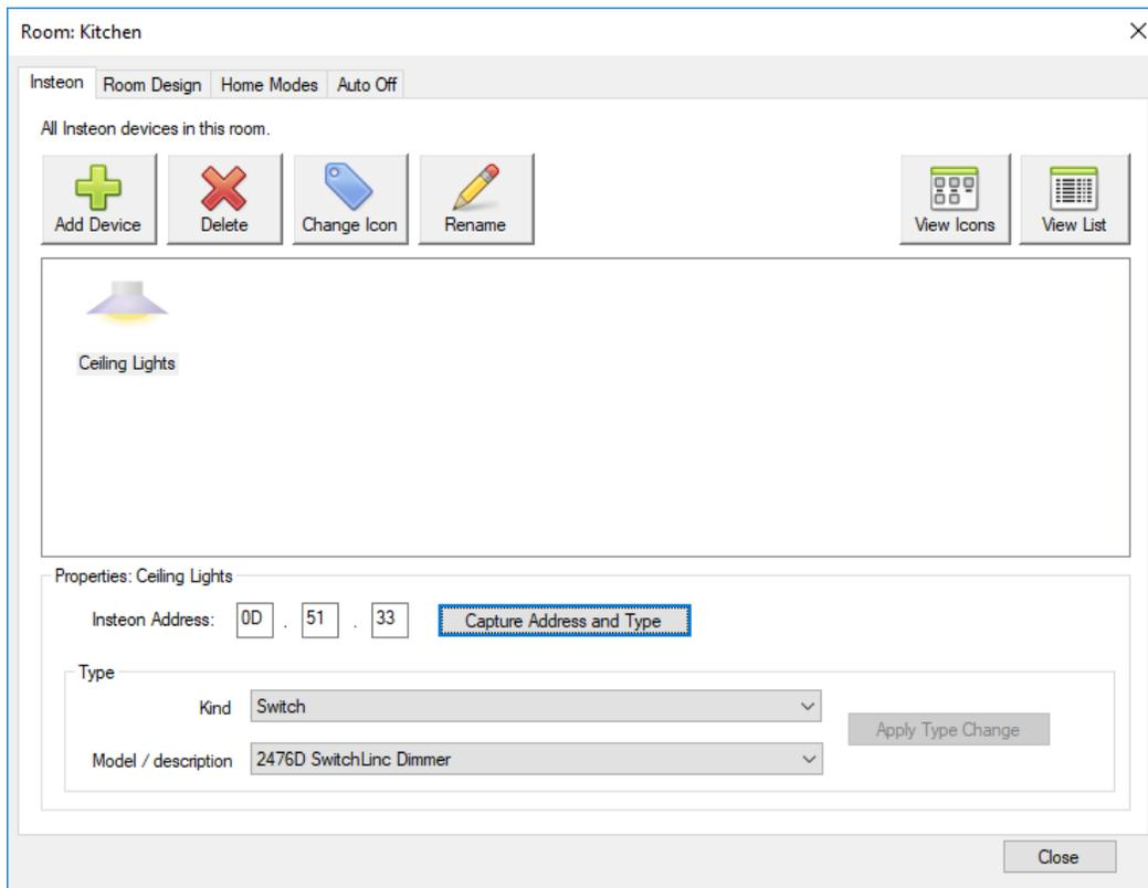
In general, there should be no reason to override the type determined unless the device is very old or a very new type, but if you need to, then select the new type with the "Kind" and "Model/description" dropdowns and then press the "Apply type change" button.
